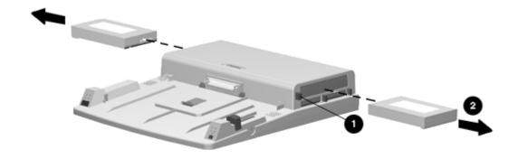
Figure 6-4. Removing a Battery Pack from a MultiBay
